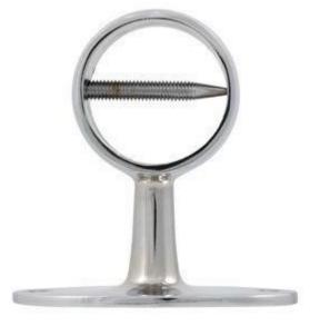
set screw. The threads of the screw will go through the rope to lock things in place. In addition, each bracket comes with two wood screws to attach it to a solid surface. These brackets accept any rope that is 1 inch in diameter. The bracket is  $2 \frac{1}{2}$  tall and the base plate is  $2 \frac{1}{2}$  x  $1 \frac{1}{2}$ .
